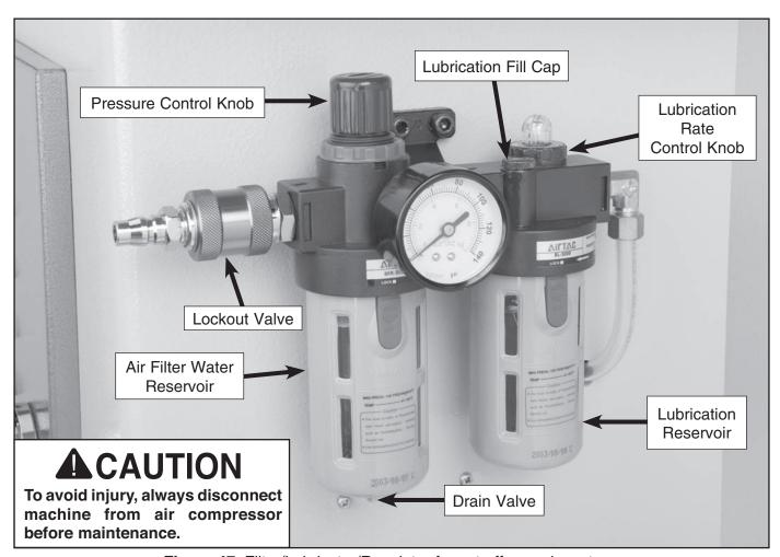
Figure 47. Filter/Lubricator/Regulator for cut-off saw air system.
